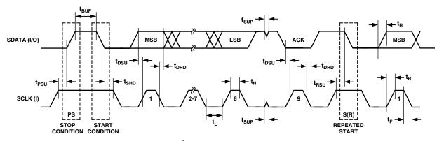
Figure 55. I<sup>2</sup>C-Compatible Interface Timing
